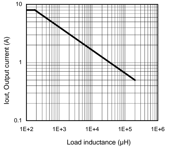
Figure 6 – Max. Output current (A) Vs Load inductance (µH)
